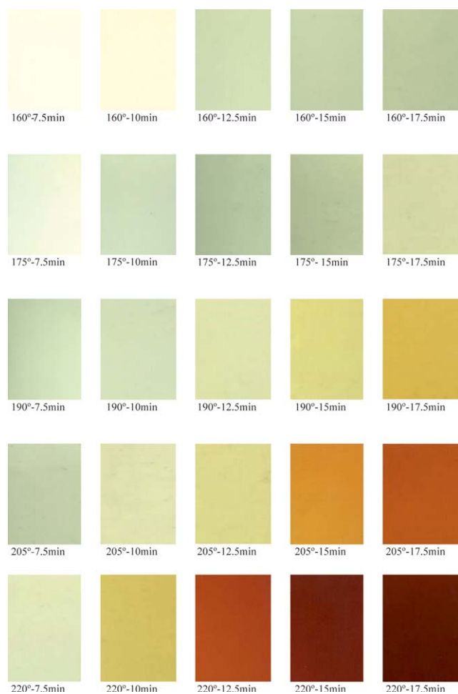
Figure 6. Optical photographs of cured PVC plastisols with ECSO plasticizer subjected to different curing conditions in terms of the isothermal curing temperature and curing time. [Color figure can be viewed in the online issue, which is available at wileyonlinelibrary.com.]
